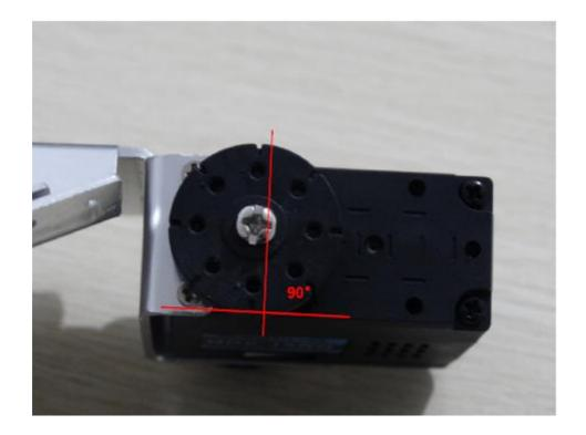
Install the front wheel as show, use M3X6 screw. Here ensure actuator state in the P1500 (previously described), ensure one hole of the steering wheel with steering gear to keep is 90 deg.
