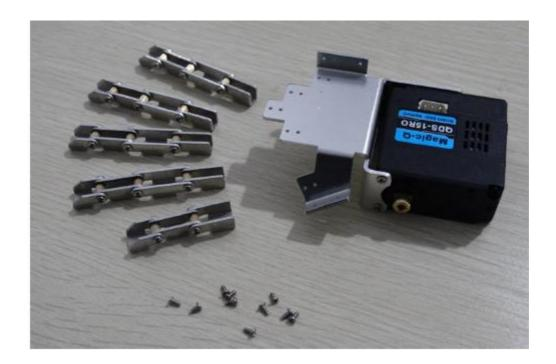
1.Install the five fingers, used M1.4X3 screw, pay attention to the assembly when the M1.4 screws as self tapping screw to force screw in the palm of the hand. Assembly as shown below
