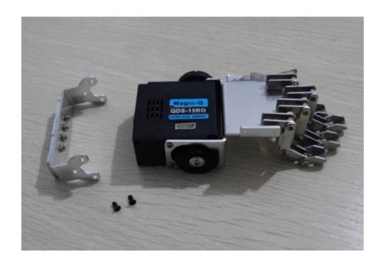
3. The installation of finger U frame, using 2\*M2X5 tapping countersunk head screw
