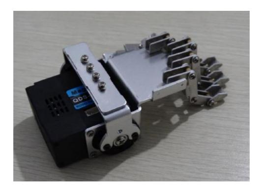
Here only install the rear steering wheel screw, **no need to install the front of the steering wheel screws**
