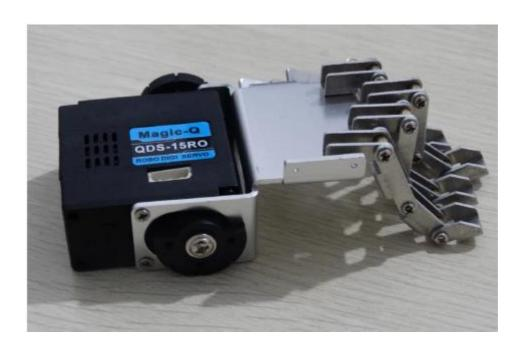
Rear rudder use M3X5 tapping countersunk head screw
