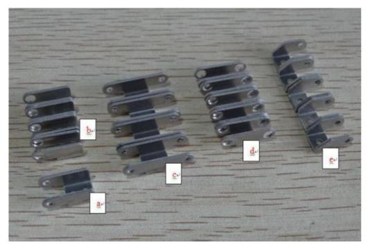
2. Assemble thumb parts as show, use M2X3 screws, M2X6 pillars.
