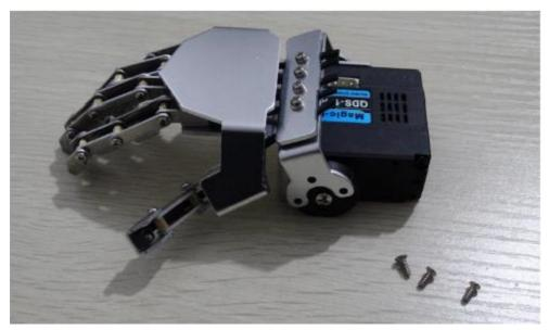
8. Pull the U bracket, this time the big finger on the index finger. Screw down the before steering wheel's 3 screws, this time must be to pull back with the U-shaped bracket, in parallel to the U frame with the actuator mounting screws.
