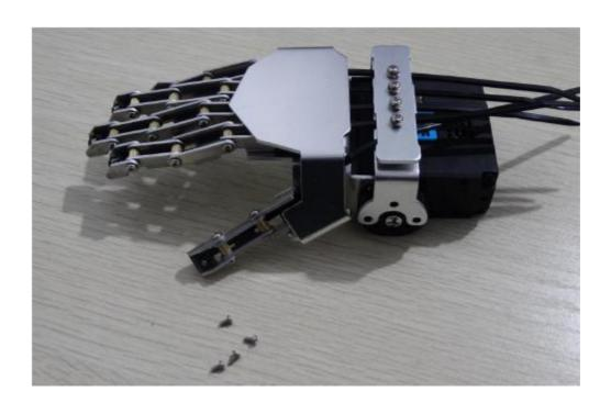
5.Cover on the back of the hand, still use the M1.4X3 screw, M1.4 screw as self tapping screws forcibly screwed into the palm of the hand.
