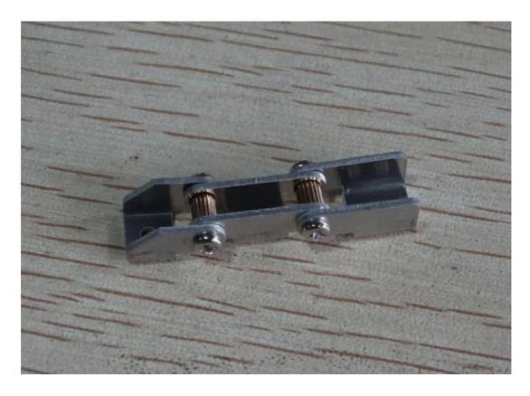
3. The other 4 fingers still use M2X3 screws, M2X6 pillars to assemble.
