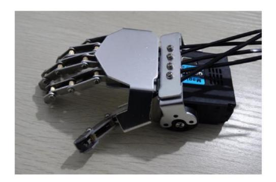
**Note** that the big finger tie loger than the other finger tie. Don't cut excess tie before adjustment over .Can push U frame back to try and ensure in the fist state the thumb above the index finger, after completing the adjustment then screw in tight.
